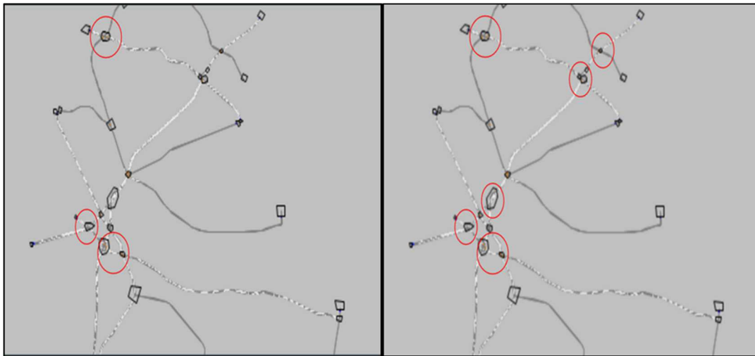
Figure 27. Bottleneck formation after announcement of Mandatory Evacuation; a) 02:00 hours of simulation (left) and b) 06:00 hours of simulation (right)
